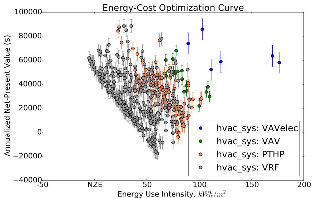
**Figure 4:** Multi-Objective Optimization Results for Commercial Office Case-Study with Economic Uncertainty (Colored by HVAC System Type)
